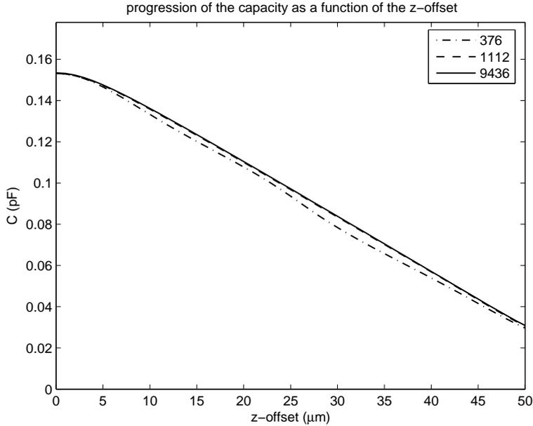
Figure 4: Capacity for centered transducers and  $\nu = 1$  (piecewise linear functions).
