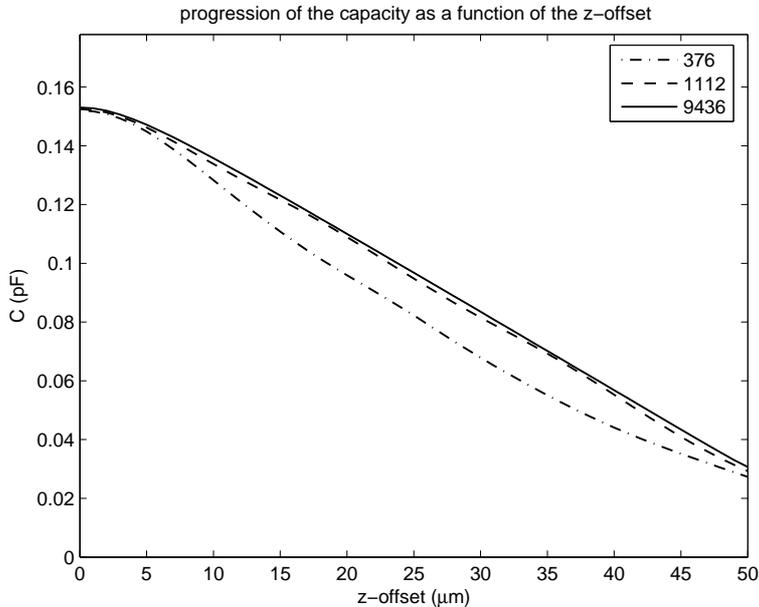
Figure 3: Capacity for centered transducers and  $\nu = 0$  (piecewise constant functions).
