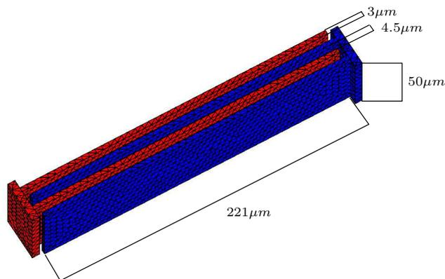
Figure 1: Geometry of a two–finger transducer.
