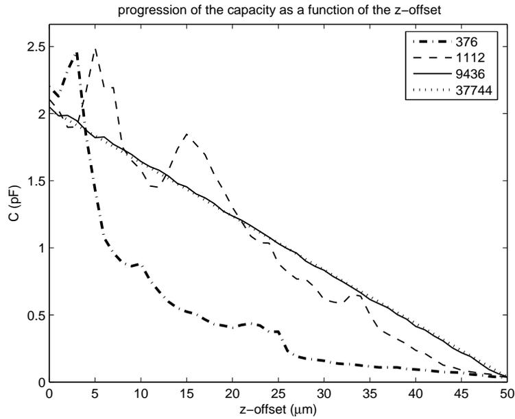
Figure 7: Capacity for transducers with small gap and  $\nu = 1$ .
