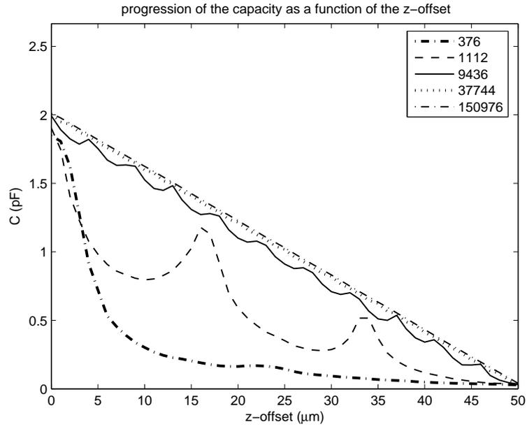
Figure 6: Capacity for transducers with small gap and  $\nu = 0$ .
